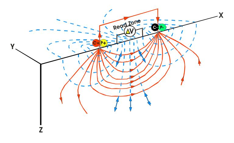
As shown in the above illustration of a two-probe array, current flows to and from the probes in all directions horizontally and vertically. As the probes are sequentially placed farther apart, the electric current goes steadily deeper. To calculate the apparent resistivity, the **EZ Res Pro** measures the voltage drop from the current sent from the **C+** and **C-** wires to the current received by the **P+** and **P-** wires. The strongest reading position is in the center of the probes.
