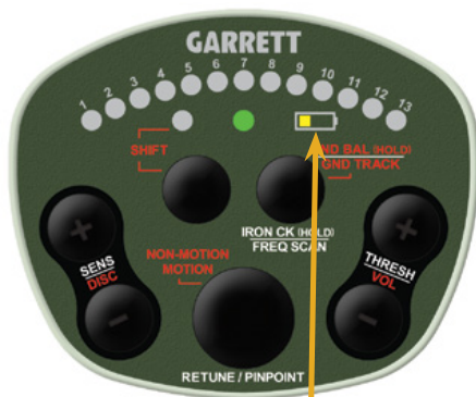
Low Battery Indicator
